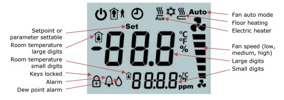
The large digits shows the measured room temperature (default setting) or the comfort setpoint (configurable via parameter P100).
