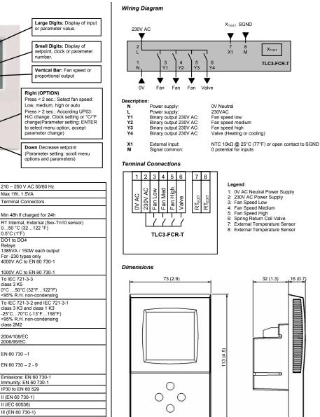
Space required in flush mounting box: (H x W x D) 60 x 50 x 32mm (2.4 x 2.0 x 1.3 in.) Distance for mounting screws: Horizontal and vertical: 45 to 63mm (1.8 to 2.5 in.)
