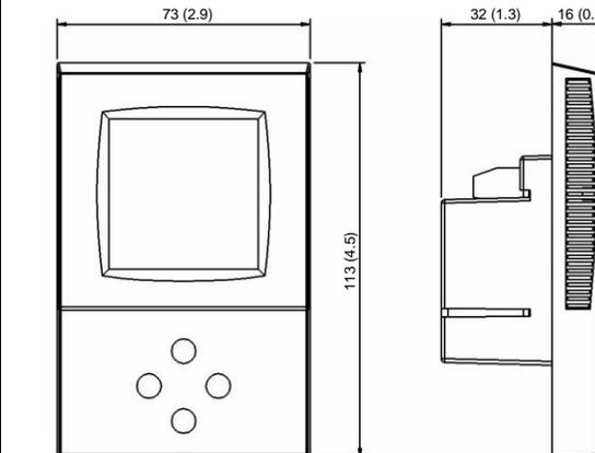
Space required in flush mounting box: (H x W x D) 60 x 50 x 32mm (2.4 x 2.0 x 1.3 in.)
