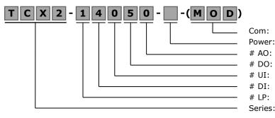
Com: Communication standard, MOD or BAC Power: Blank = 24VAC, 230 = 230VAC # AO: 0 Analog outputs # DO: 5 Binary outputs # UI: 0 Analog inputs # DI: 4 Passive inputs # LP: 1 control loops Series: **TCX2**
