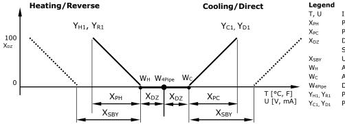
Input signal temp/universal P-band heating/direct P-band cooling/reverse Dead zone between displayed SP and acting SP in 4-pipe mode Unoccupied mode set point shift Acting set point heating/reverse Acting set point cooling/direct Displayed set point in 4-pipe mode PI sequence heating/reverse PI sequence cooling/direct
