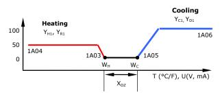
increases until it reaches the maximum heating output (1A04), typically 30 to 50% of maximum cooling airflow.
