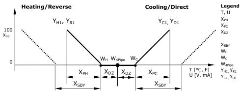
Input signal temp/universal P-band heating/direct P-band cooling/reverse Dead zone between displayed SP and acting SP in 4-pipe mode Unoccupied mode set point shift Acting set point heating/reverse Acting set point cooling/direct Displayed set point in 4-pipe mode PI sequence heating/reverse PI sequence cooling/direct
