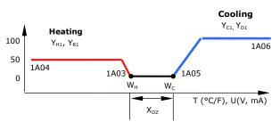
increases until it reaches the maximum heating output (1A04), typically 30 to 50% of maximum cooling airflow.
