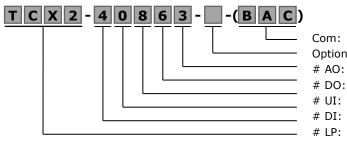
Com:Communication standardOption:OP = with operation terminal# AO:3 Analog outputs# DO:6 Binary outputs
