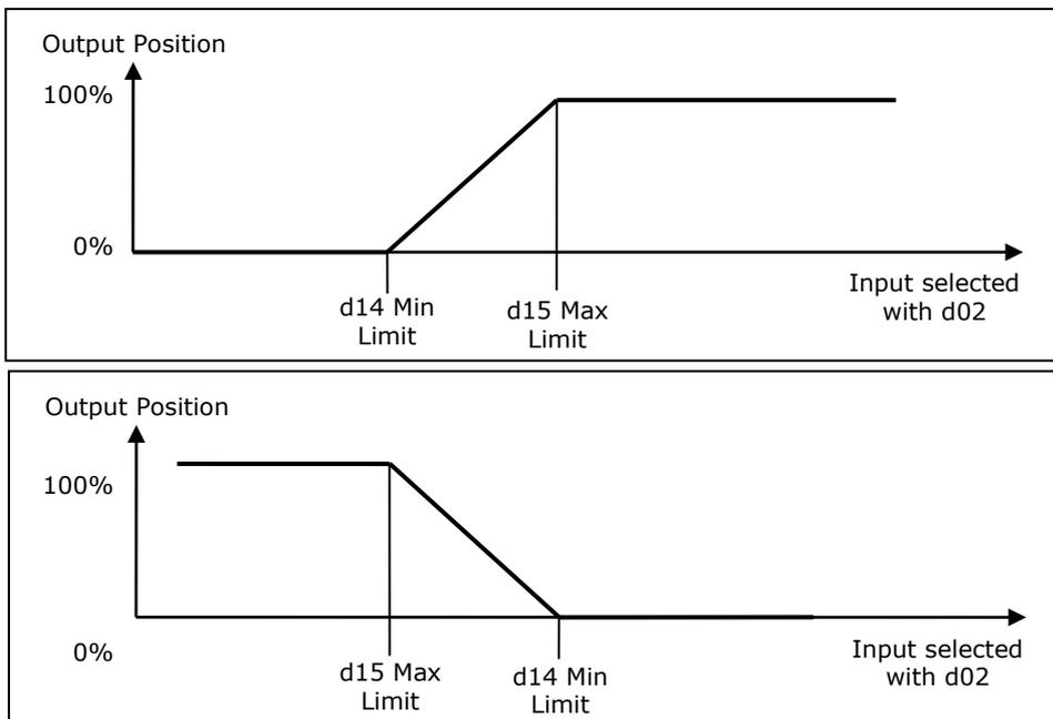
**Parameter reference for floating output configuration**
