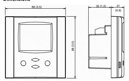
Space required in flush mounting box:  $(H \times W \times D)$
