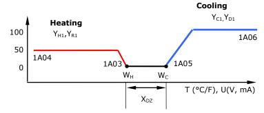
reaches the maximum heating output (1A04), typically 30 to 50% of maximum cooling airflow.
