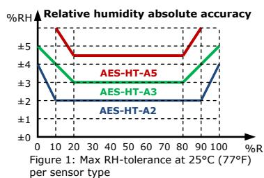
Note on accuracy: Allow 1 hour after power up for compensation swing in until described accuracy is reached.
