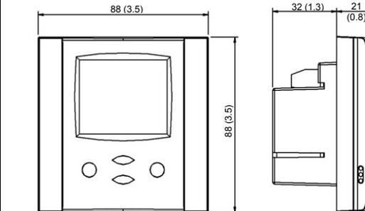
Space required in flush mounting box: (H x W x D) 60 x 50 x 32mm (2.4 x 2.0 x 1.26 in.)
