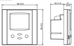
Space required in flush mounting box: (H x W x D) 60 x 50 x 32mm (2.4 x 2.0 x 1.3in.)
