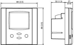
Space required in flush mounting box: (H x W x D) 60 x 50 x 32mm (2.4 x 2.0 x 1.3 in.) Distance for mounting screws: Horizontal and vertical: 45 to 63mm (1.8 to 2.5 in.)
