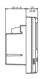
Space required in flush mounting box: (H x W x D)  $60 \times 50 \times 32$ mm (2.4 x 2.0 x 1.26 in.)
