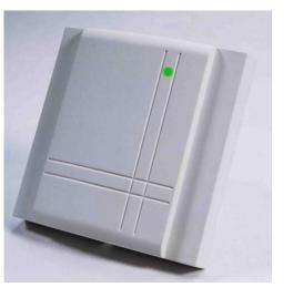
The CO2 concentration is measured through non-dispersive infrared (NDIR) waveguide technology with ABC automatic background calibration algorithm. The applied measuring technology guarantees excellent reliability and long-term stability. The microprocessor samples the CO2 once per second. It calculates an averaging signal over a preset number of seconds and generates the output signal.
