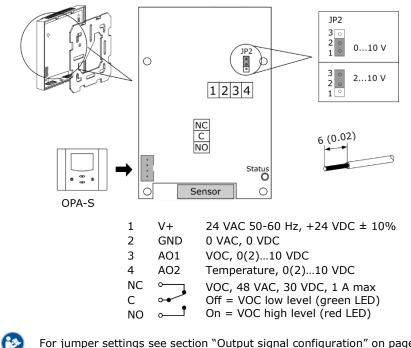
For jumper settings see section "Output signal configuration" on page 5.
