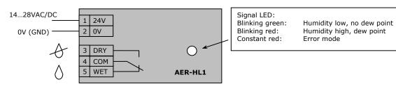
DRY = When the device is powered and no dew point alarm is active WET = When the device is not powered or a dew point alarm is active
