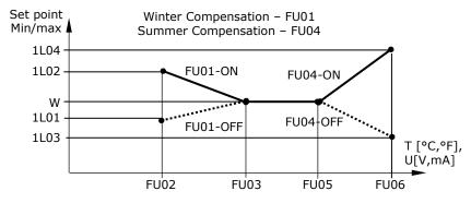
→ Use occupied (comfort)/unoccupied (economy) mode changeover with key card switches, occupancy sensors, etc. Set input limit 1 and 2 with possibilities below. Example: When Limit 2 is greater than Limit 1, switch comfort-to-economy at the lower value, economy-to-comfort at the higher value. Activate occupied (comfort)/unoccupied (economy) changeover with loop configuration parameter(LO7).
