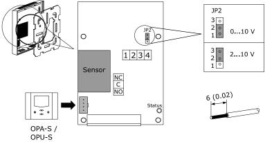
V+ AC 24 V 50-60 Hz, DC +24 V  $\pm$  10% 1 2 **GND** AC 0 V, DC 0 V 3 AO1 CO2, DC 0(2)...10 V 4 AO2 Temperature, DC 0(2)...10 V NC CO2, 48 VAC, 30 VDC, 1 A max С Off = CO2 low level (green LED) NO On = CO2 high level (red LED)
