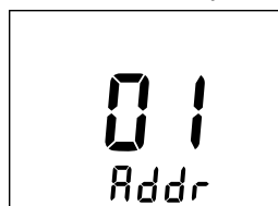
Modbus address (example)
