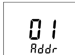
Set Modbus address menu (alternating)
