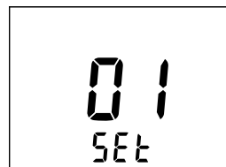
Set Modbus address menu (alternating)
