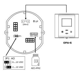
(i) NOTE: For parameter programming, the OPA-S programming and display unit must be plugged in at the connector under the front panel or on the back of the MZ3.
