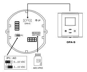
NOTE: For parameter programming, the OPA-S programming and display unit must be plugged in at the connector under the front panel or on the back of the MZ3.
