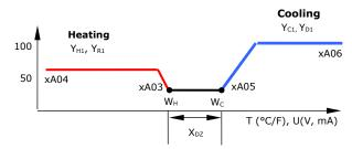
increases until it reaches the maximum heating output (A04), typically 30 to 50% of maximum cooling airflow.
