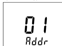
Set Modbus address menu (alternating)
